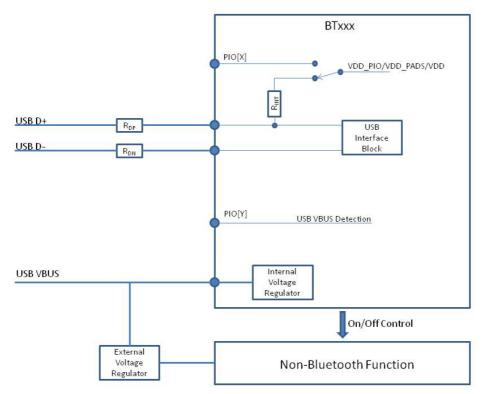
Figure 4: High-power bus-powered BTxxx device
