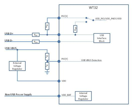
Figure 5: Self-powered WT32 device
