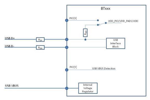
Figure 2: Low-power bus-powered BTxxx device configuration
