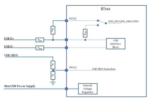
Figure 7: Self-powered BTxxx device
