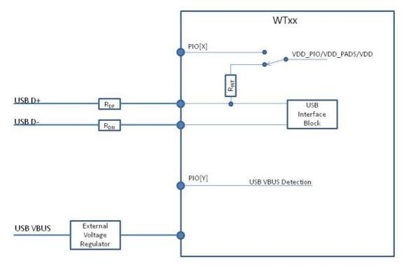
Figure 1: Low-power bus-powered WTxx device configuration
