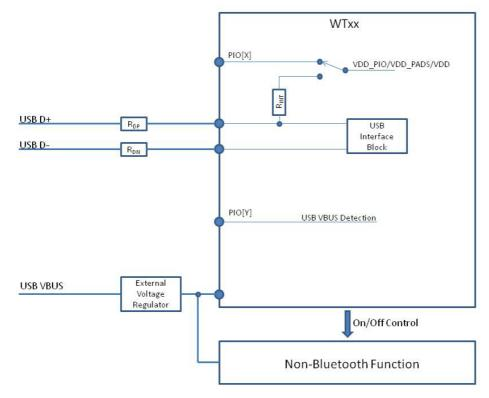
Figure 3: High-power bus powered WTxx device
