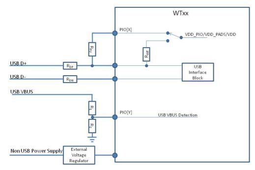
Figure 6: Self-powered WTxx device
