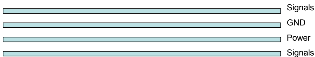
Figure 1: Typical 4-layer PCB construction
