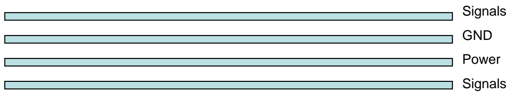
Figure 8: Typical 4-layer PCB construction
