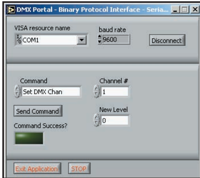
Photo 2 —Using LabVIEW, it is easy to create utilities that communicate over standard PC I/O ports and have professional-looking graphical user interfaces. This utility allows the DMX Portal to be accessed through the RS-232 interface using the binary protocol.
