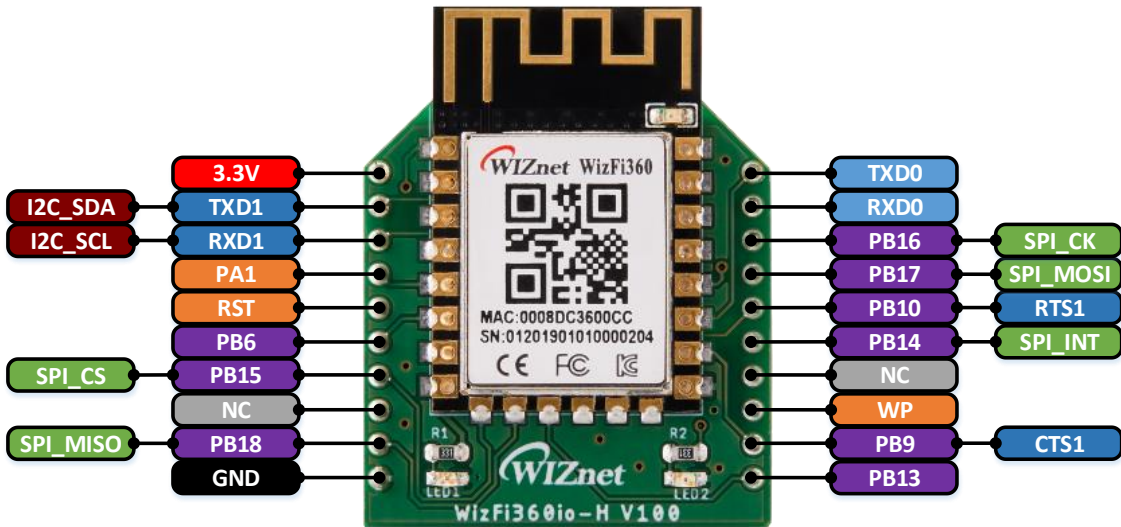
Figure 2. WizFi360io-H Pinout
