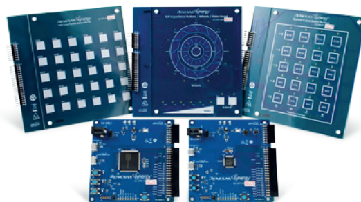
Figure 12-3: The AE-CAP1 provides everything needed to develop a touch sensor application
