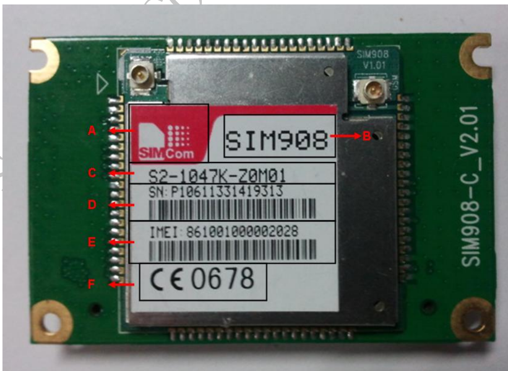
Figure 41: Top view of SIM908-C
