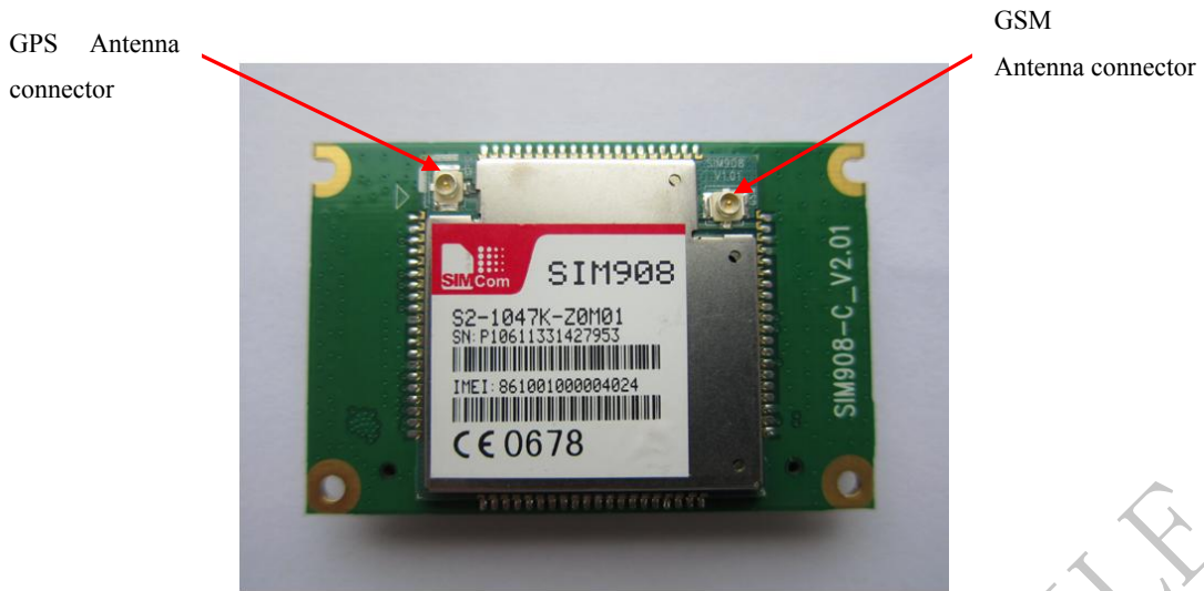
Figure 38: The RF interface of module
