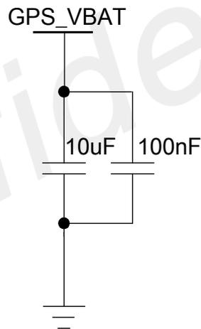
Figure 40: Reference circuit of the GPS\_VBAT input
