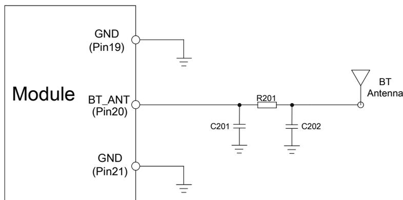
**Figure 39: Bluetooth antenna matching circuit**
