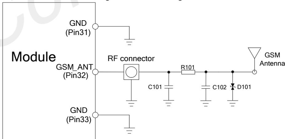
**Figure 37: GSM antenna matching circuit**
