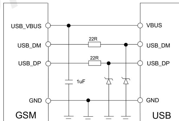
**Figure 23: USB reference circuit**
