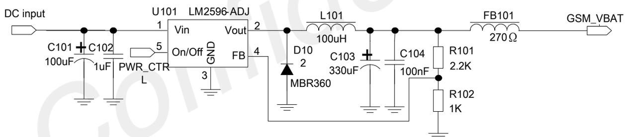
**Figure 11: Reference circuit of the DC-DC power supply**
