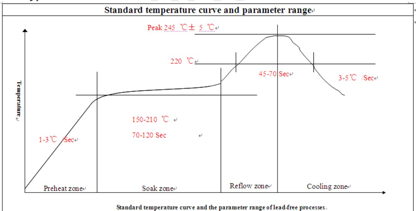
Figure 53: Typical solder reflow profile of lead-free process
