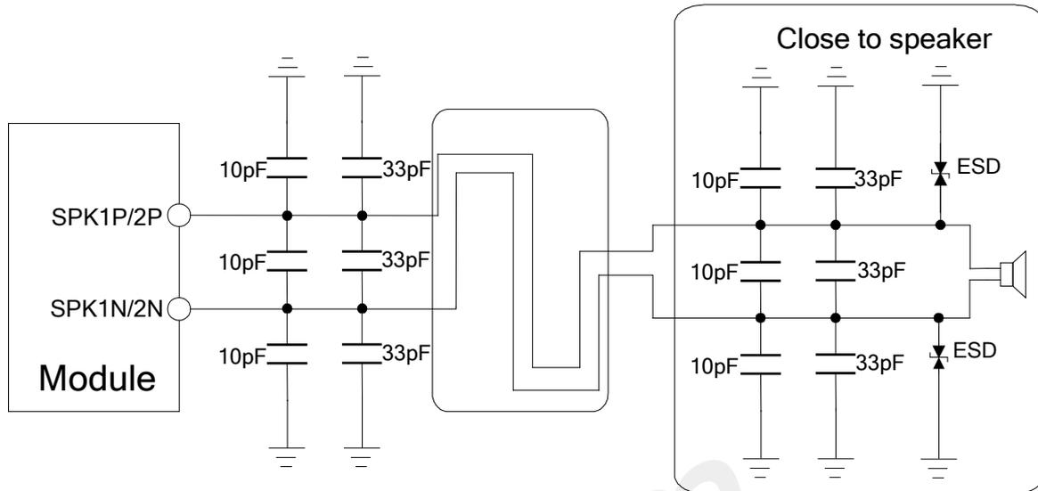
Figure 28: Speaker reference circuit
