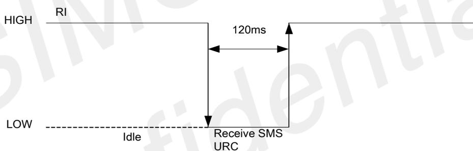
**Figure 26: UART1\_RI behaviour of URC or receive SMS**
