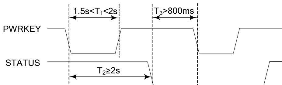
Figure 17: Timing of restart GSM
