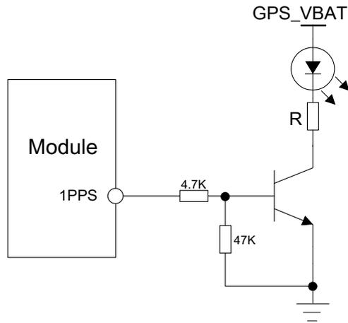
**Figure 48: 1PPS Application circuit**
