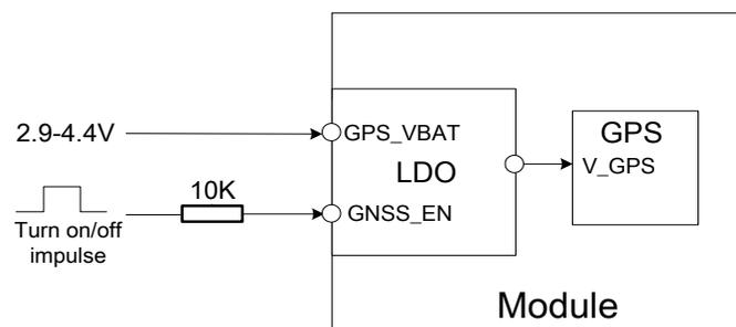
Figure 43: Power on/off GNSS
