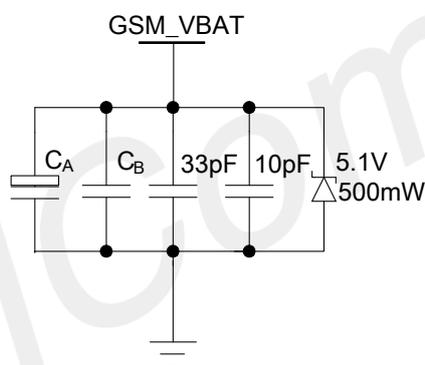
**Figure 8: Reference circuit of the GSM\_VBAT input**
