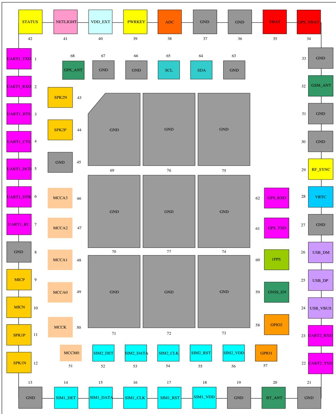
**Figure 51: PIN assignment**
