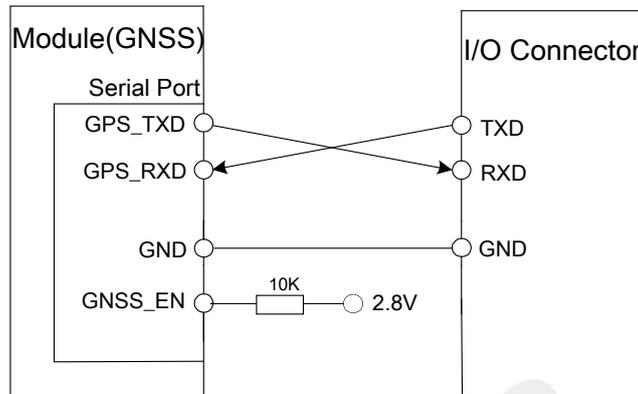
**Figure 46: Connection for software upgrading and debugging for GNSS**
