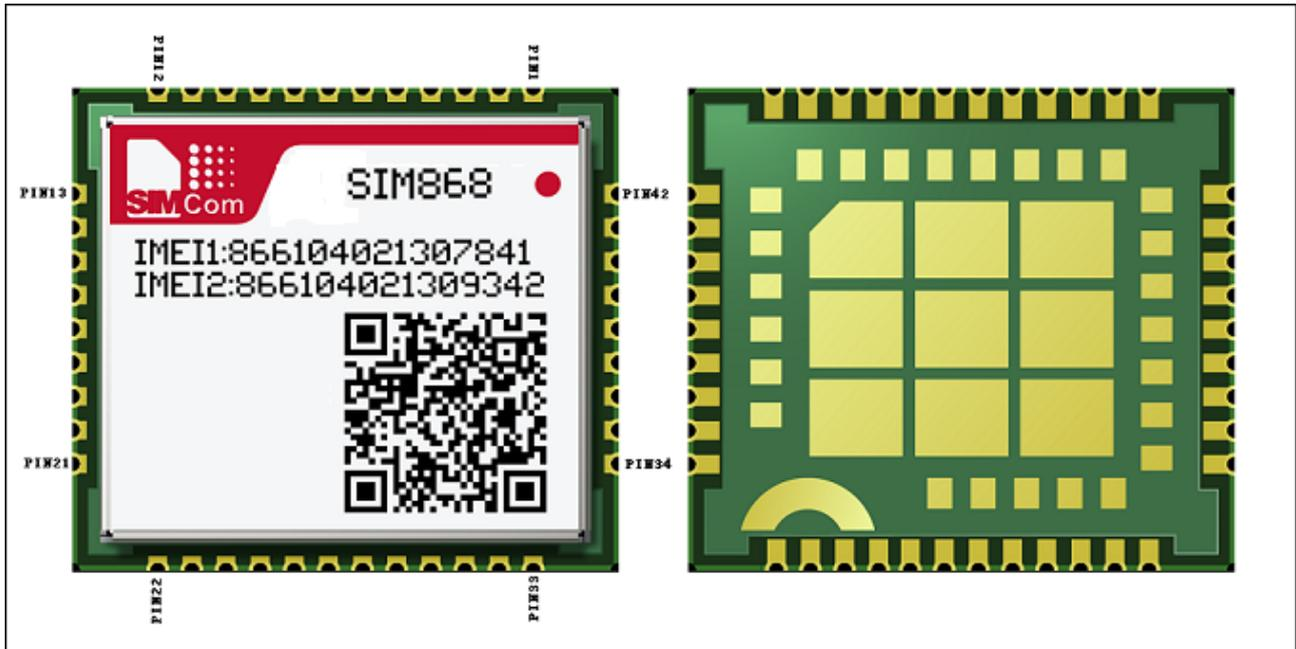
Figure 52: Top and bottom view of SIM868
