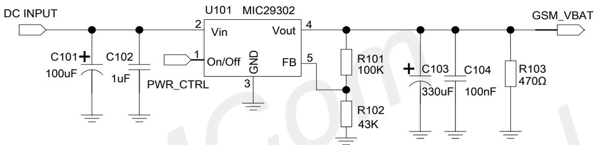
**Figure 10: Reference circuit of the LDO power supply**
