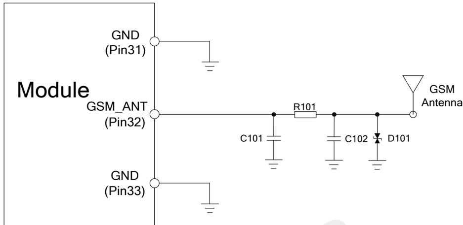
**Figure 38: GSM antenna matching circuit without RF connector**
