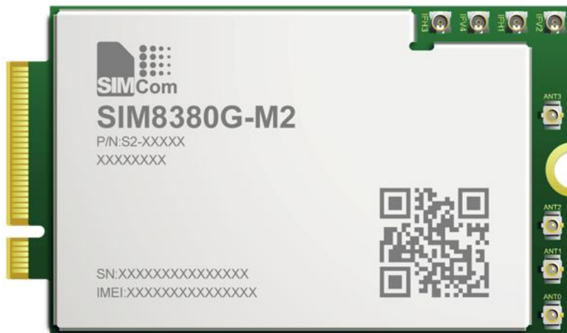
Figure 37: Antenna interfaces of Modules
