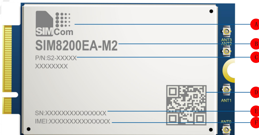
Figure 37: Label description of the module
