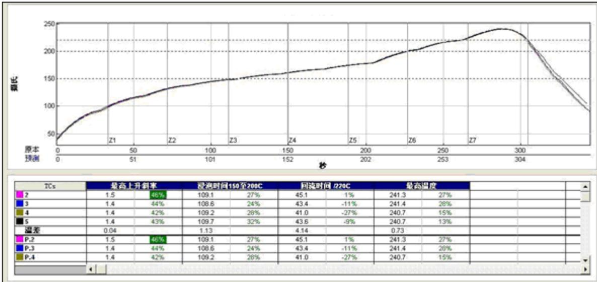
Figure 14: The Ramp-Soak-Spike reflow profile of SIM68R
