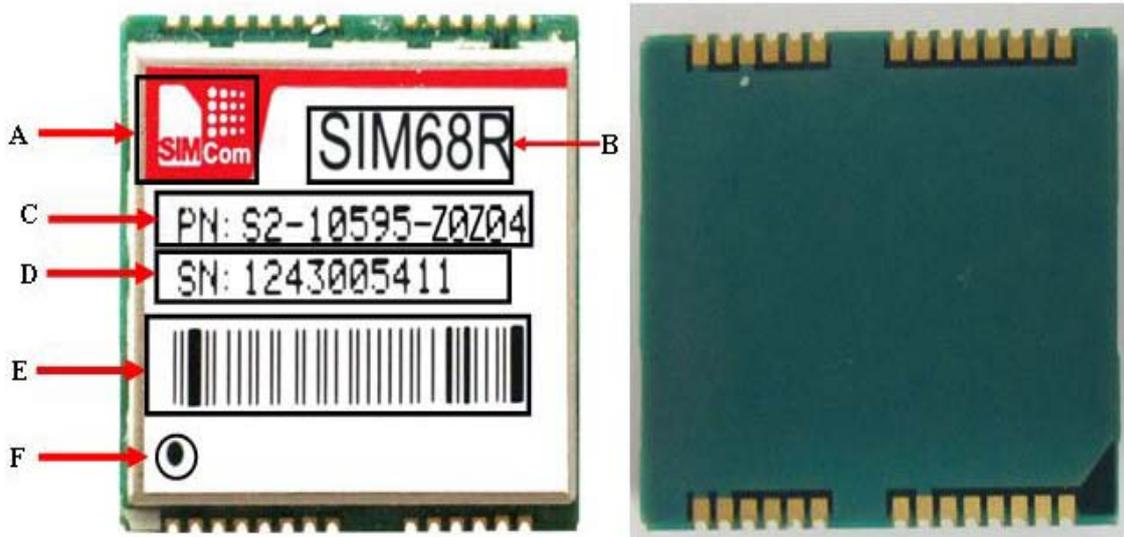
Figure 13: Top and bottom view of SIM68R
