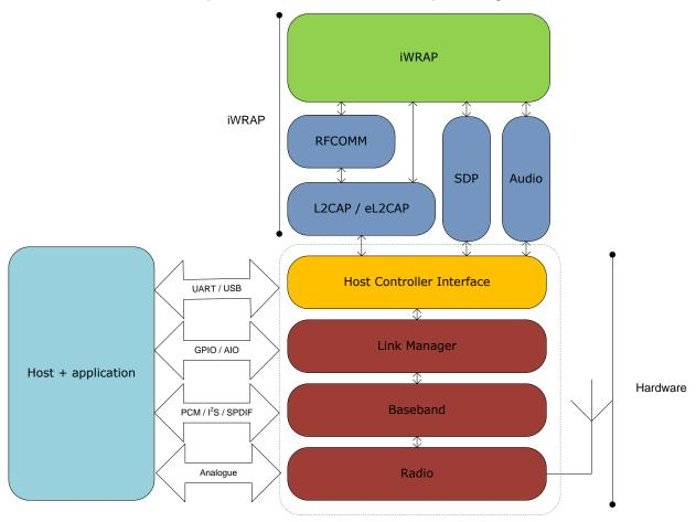
Figure 1: iWRAP Stack
