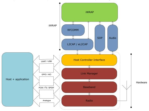
Figure 2: iWRAP Bluetooth stack
