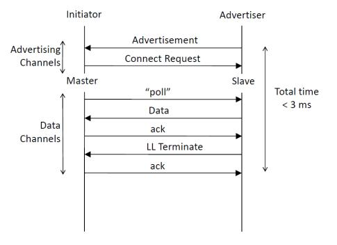
10ms connection interval + ACK allow data to be sent every 20ms. At 20B payload this is about 1000B/sec.
