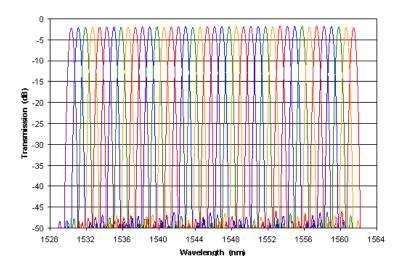
Typical Moderrate 40-Channel Spectrum
