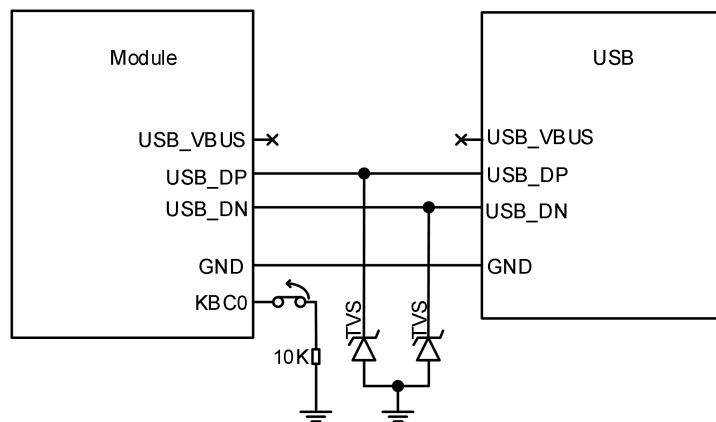
Figure 21: Forced download reference circuit for SIM800
