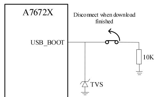
Figure 23: Forced download reference circuit for A7672X
