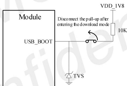
Figure 22: Forced download reference circuit for A7670E
