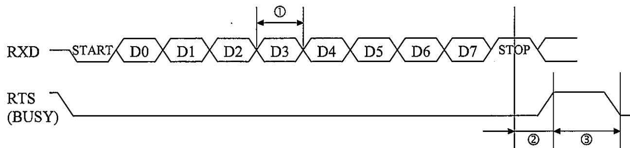
$$\textcircled{1} \quad t(\text{DATA}) = 10^6 / 9600(\text{bps}) [\mu\text{s}]$$
