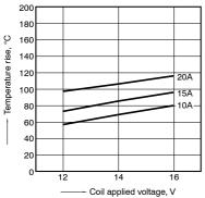
1-(4). Coil temperature rise (at 85°C 185°F) Sample: ACJ2212, 3pcs Measured portion: Inside the coil
