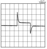
2-(2). Electrical life test (Motor lock) Sample: ACJ2212, 3pcs; Load: Steady current: 25A, Power window motor actual load (lock condition); Tested voltage: 14V DC; Switching frequency: (ON:OFF = 0.5s:9.5s); Switching cycle: 10<sup>5</sup>; Ambient temperature: Room temperature Circuit
