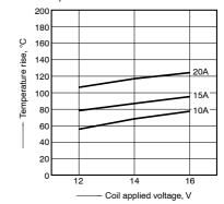
1-(6). Coil temperature rise (at 85°C 185°F) Sample: ACJ5212, 3pcs Measured portion: Inside the coil
