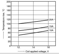
1-(2). Coil temperature rise (at 85°C 185°F) Sample: ACJ1212, 3pcs Measured portion: Inside the coil Contact carrying current: 10A, 15A, 20A
