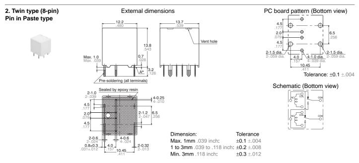
\* Dimensions (thickness and width) of terminal specified in this catalog is measured before pre-soldering. Intervals between terminals is measured at A surface level.
