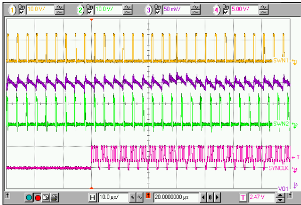
Top to Bottom: SWN_Slave, Vo_Slave, SWN_Master, Sync_clk
