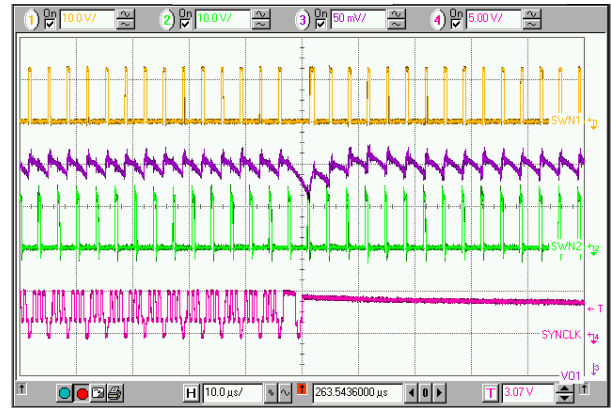
Top to Bottom: SWN_Slave, Vo_Slave, SWN_Master, Sync_clk
